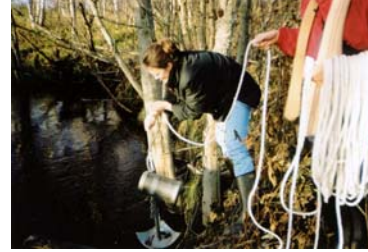
Stormwater sampling with SPMD
