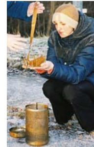
Stormwater sampling with SPMD
