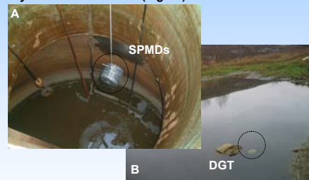
Figure 1. A: SPMD deployment into the leachate reservoir; B: DGT deployed in leachate dam
